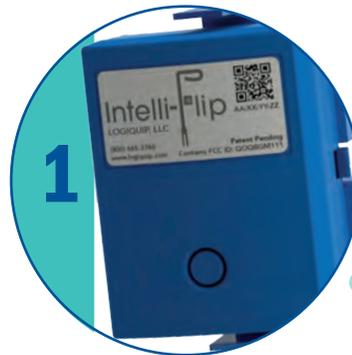
1 The Intelli-Flip Monitor is attached to the Kanban Divider. A signal is sent to the Controller when accessing safety stock.
